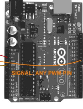
NOTE: This motor may need more power than is available from a standard USB port. If you attempt to use your SG90 Micro Servo powered solely by USB, the motors may stutter and fail. To fix this simply plug the board into a wall socket, or battery.
