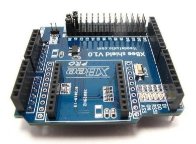
XBee Shield V1.0 is an enhanced serial port XBee module breakout board, it's compatible with Arduino and IFLAT-32, it can directly plug in with Arduino/IFLAT-32 board, and use any pin of the basic board to connect with the XBee module serial port.
