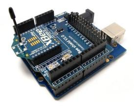
This shield provides 3 optional hardware interfaces for Arduino wireless program.
